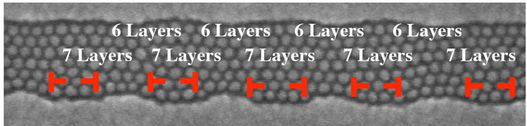
Demonstration of control of ordering and introduction of defects within confined block-copolymers. SEM image by Dr. Joy Cheng, MIT.
